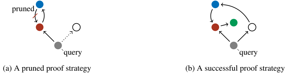
Figure 8: Proof diagrams showing two strategies for proving a query. Nodes represent premises. Edges represent proof dependencies; unexplored edges are dotted. In strategy (a), the proof search for the blue node is pruned because its proof depends on the red node, which would introduce a cycle in the proof diagram. Strategy (b) results in a successful proof: the proof forms a DAG, wherein all leaf nodes are axioms.
